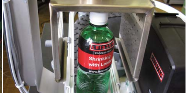
HOTWIND SYSTEM as hot air provider in a shrinking process.
